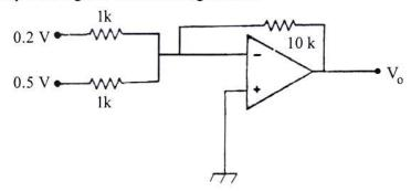
(d) Find out the output voltage of the following two circuits:
